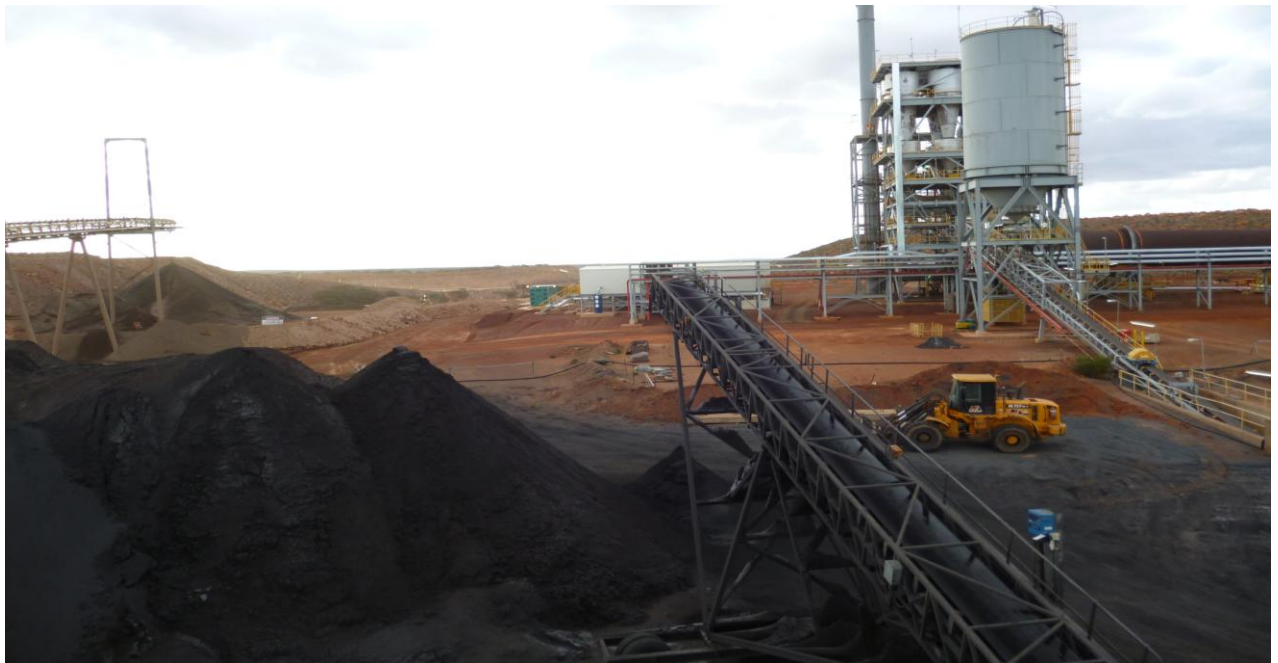
Stockpiled magnetite concentrate ready for roasting in the kiln
